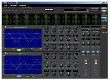
If two bands are set to the same frequency, the gain settings are additive and the response curve may go off the display. The response is not limited to the display scale, and the 32-bit floating-point processors accurately calculate the combined response of all five bands.
